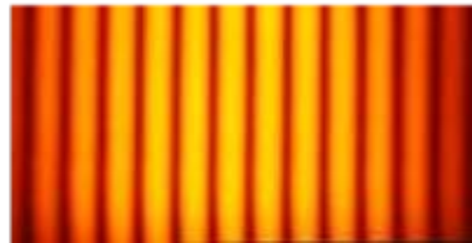
Figure 3: Interference patterns formed by scanning the optical path difference of a monochromatic light in Michelson Interferometer (Wikipedia Creative Commons Attribution-Share Alike 4.0 International license)
